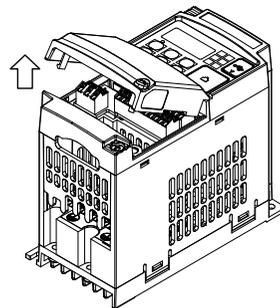
(3) Connect wires of WJ-VL to the control logic terminal.
