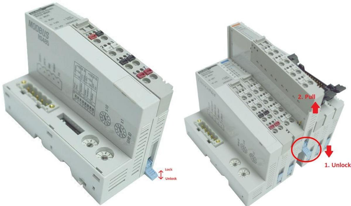
As above figure in order to safeguard the FnIO module from jamming, it should be fixed onto the DIN rail with locking level. To do so, fold on the upper of the locking lever. To pull out the FnIO module, unfold the locking lever as below figure.
