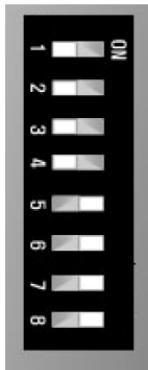
MODBUS Adapter interface configuration can be set by a DIP (8pole) switch. This setup read once at power-up sequence, i.e. changes to DIP switch during operation does not affect MODBUS interface configuration.
