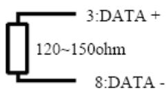
A reflection in a transmission line is the result of an impedance discontinuity that a traveling wave sees as it propagates down the line. To minimize the reflections from the end of the RS485-cable it is required to place a Line Termination near each of the 2 Ends of the Bus.
