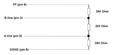
In order to minimize cable reflections and ensure a defined noise level on the data lines,
