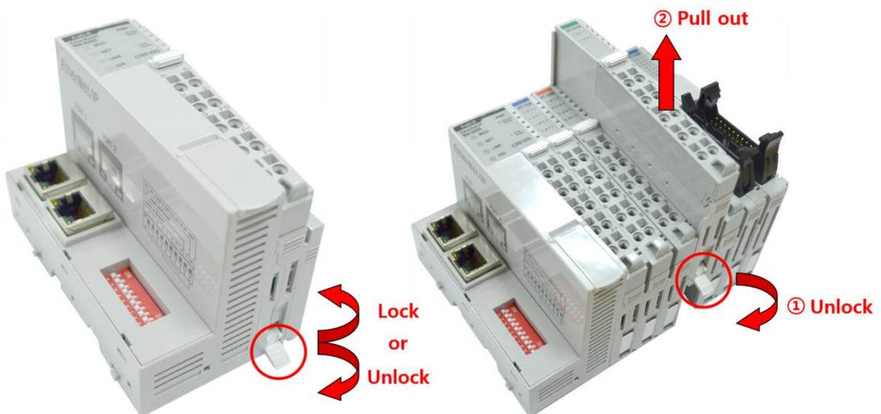
As above figure in order to safeguard the RIO3 module from jamming, it should be fixed onto the DIN rail with locking lever. To do so, fold on the upper of the locking lever.
