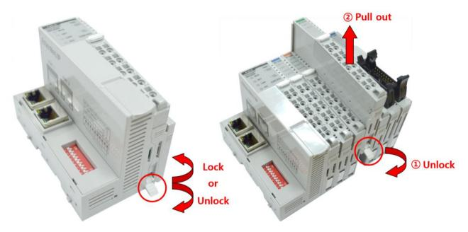
As above figure in order to safeguard the RIO3-Module from jamming, it should be fixed onto the DIN rail with locking lever. To do so, fold on the upper of the locking lever.
