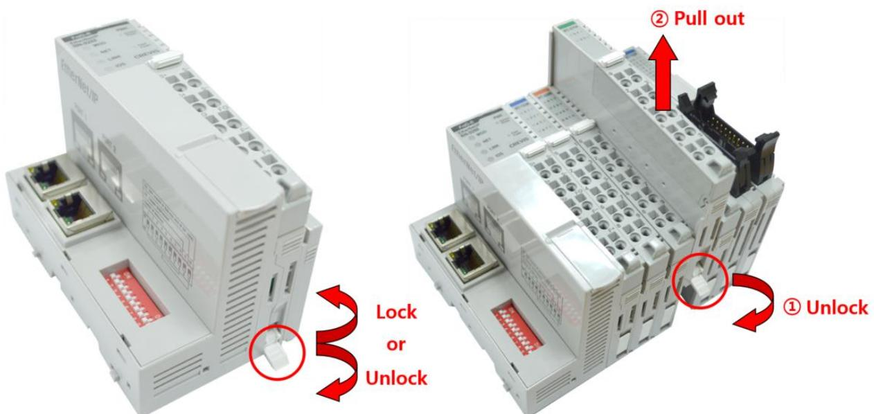
As above figure in order to safeguard the RIO3-Series module from jamming, it should be fixed onto the DIN rail with locking lever. To do so, fold on the upper of the locking lever.
