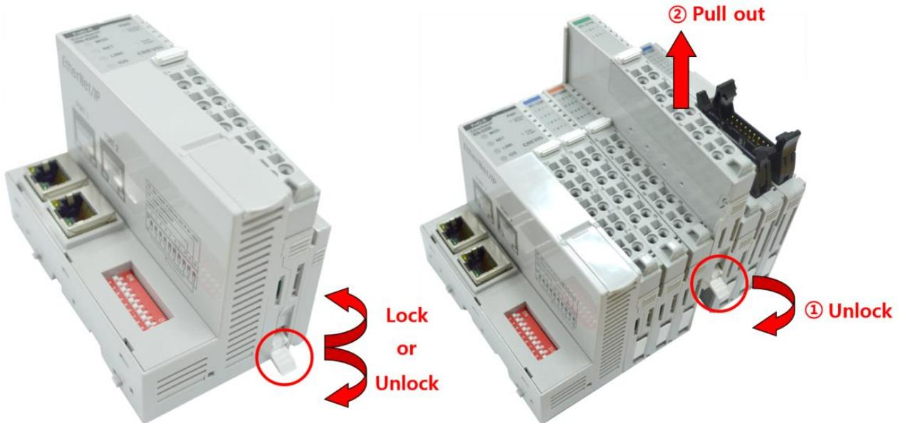
As above figure in order to safeguard the RIO3-Module from jamming, it should be fixed onto the DIN rail with locking level. To do so, fold on the upper of the locking lever.
