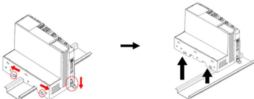
As above figure in order to safeguard the RIO3 module from jamming, it should be fixed onto the DIN rail with locking level. To do so, fold on the upper of the locking lever. To pull out the RIO3 module, unfold the locking lever as above figure.
