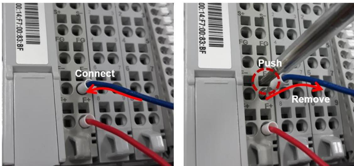
Connecting or removing the cable by pushing the terminal button for the relevant points.
