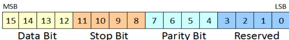
\*\*Modbus Station : This description for 0x160A register with bit.
