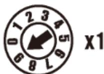
Each MODBUS Adapter could have an unique address (from 1 to 99) so that it can be addressed independently from other nodes. The address 0 is reserved to identify a broadcast exchange. No response is returned to broadcast requests sent by the master.
