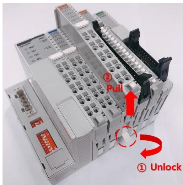
As above figure in order to safeguard the RIO3 module from jamming, it should be fixed onto the DIN rail with locking lever. To do so, fold on the upper of the locking lever. To pull out the RIO3 module, unfold the locking lever as below figure.
