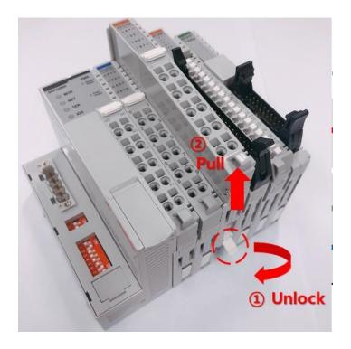
As above figure to safeguard the RIO3 module from jamming, it should be fixed onto the DIN rail with locking level. To do so, fold on the upper of the locking lever. To pull out the RIO3 module, unfold the locking lever.
