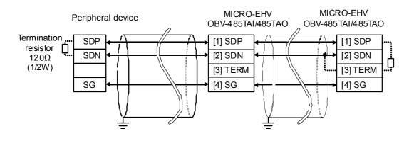
Use the built-in termination resistor (120 $\Omega$ ) in OBV-NES / 485A / 485TAI / 485TAO depending on the usage environment and communication cable.
