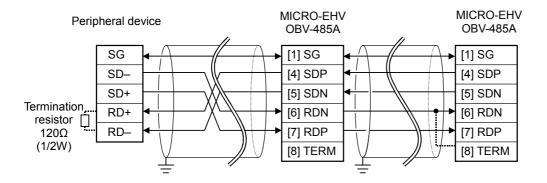
The example of the cable connection of RS-485 I/F is shown below. Be sure to use shielded twisted pair cable.
