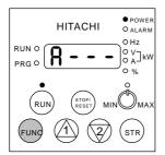
Make monitor display "A - - -" by referring to (1) displaying method.
