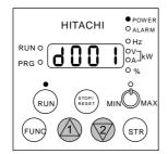
Monitor mode is displayed by pushing FUNC (Function) key once when display of Monitor mode No.
